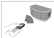
Place the RF remote control near the sensor (within two inches) and press the 0 key on the remote until the red LED on the sensor illuminates. Repeat with other RF remote controls (up to four).
