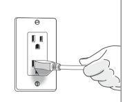
Plug the power strip into a grounded receptacle. The ground and surge lights will illuminate - indicating proper grounding and surge protection is functional.
