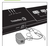
Plug the multi-sensor into the port on the side of the power strip that looks like a phone jack.
