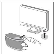
Remove the backing from the double sided tape on the back of the multi-sensor & affix to or near the TV.
